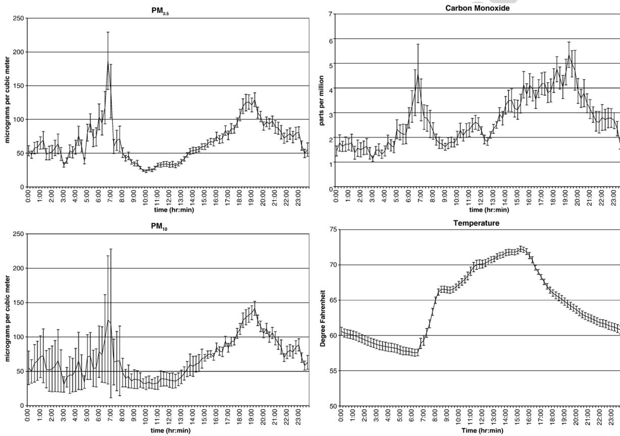
Fig. 2. 15-minute mean  $\pm 1$  standard error PM<sub>2.5</sub>, PM<sub>10</sub>, CO and temperature present at the Session Road monitoring station throughout the entire sampling period ( $n=11$  days).
